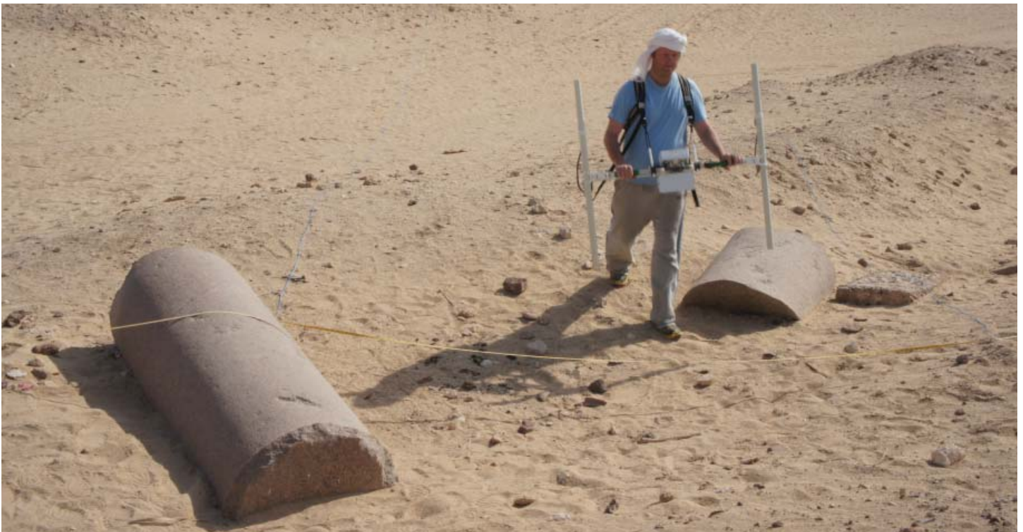
Top: L to R, Omar, Khaled, Waleed & Kris laying out 30-meter grid squares for magnetometry. Bottom: Kris taking measurements with magnetometer in Test Area 4.
